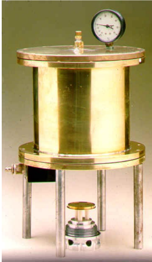
Frisch Grid ionization chamber designed in 1959 by Elizabeth Rona
